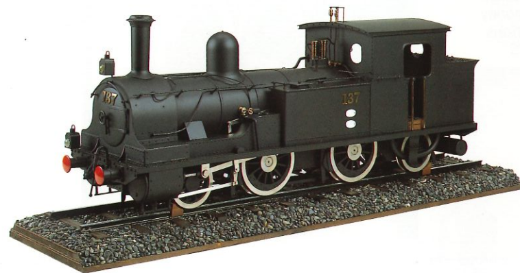
③ Japan's first domestically-built steam locomotive (scale model), was built in 1893 at the Railway Agency's Kobe factory under the guidance of an English engineer.
